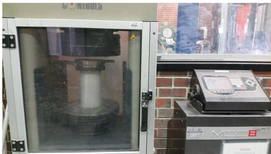
Figure 3.11 Compressive strength test setup for concrete specimens.
