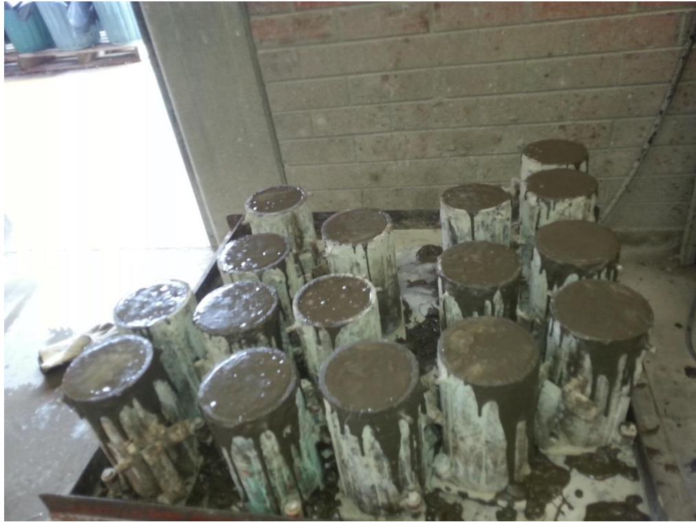
Figure 3.3 Cylinders mould after compaction
