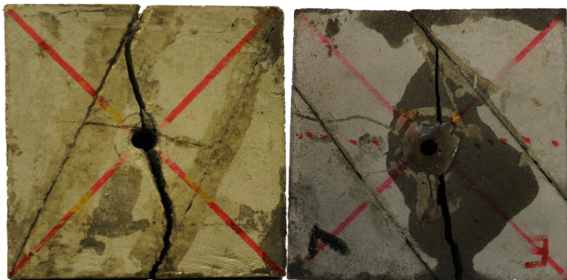
Figure 3.31 Opening interaction that happened in hydraulic fracturing propagating toward the strong brittle interface in low angle of approach in 10 cm samples.
