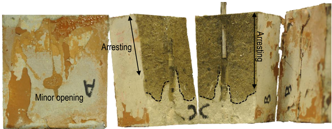
Figure 3.37 Hydraulic fracturing experiment conducted on the sample of 10 cm cube of cement having two orthogonal brown-glued interfaces. The fracture has arrested by both of interfaces. A small opening section is observed on the left hand side interface.
