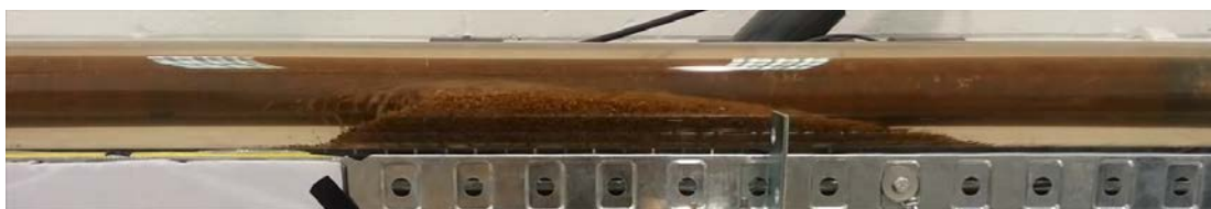
Figure 4.23 Dune movement of cuttings in Fluid #1 (water)
