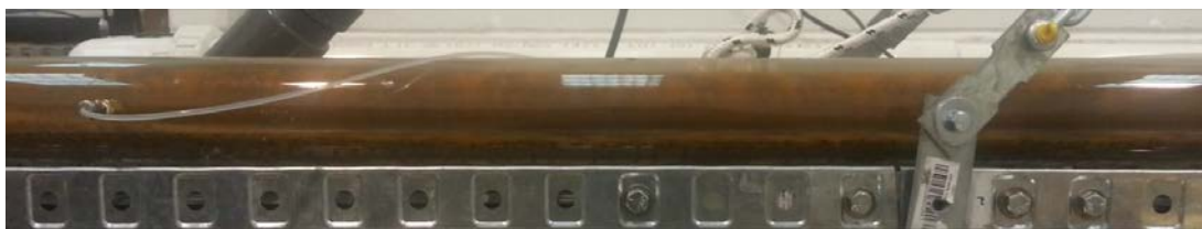
Figure 4.24 Stationary/moving bed of cuttings in Fluid #2
