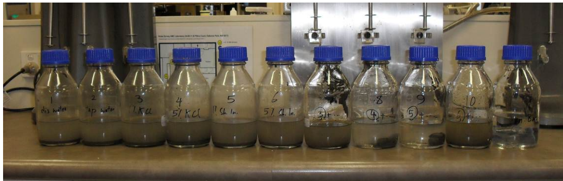
Figure A.2 Adding 20g of cuttings to the fluid samples
