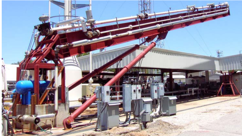
Figure 2.9 The drilling section of the ACTF at an inclination of 25° (Miska et al., 2004)
