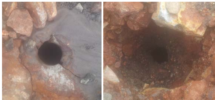
Figure 6.1 The wells drilled with a hammer bit. Left: without washout, right: with washout
