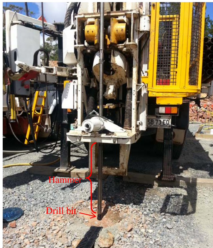
Figure A.3 The Wassara downhole hammer connected to the drill bit
