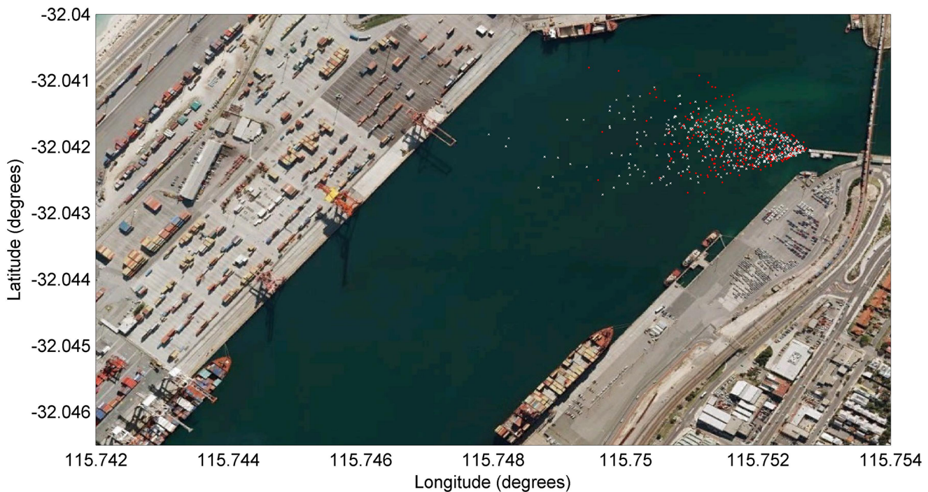
Fig 5. Position of first detected dolphin within a group in the Fremantle Inner Harbour as a function of range and bearing using both cameras. White dots correspond to plots obtained from the still camera and red dots correspond to plots obtained from the video camera.
