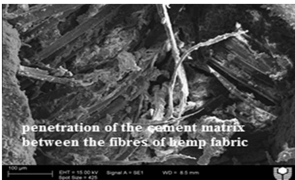
Fig. 5. Penetration of the cement matrix in between the reinforced fibres of hemp fabric.
