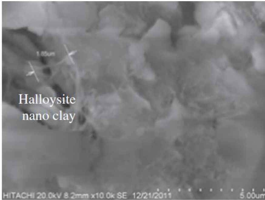
Figure 2.45: Cross-linking effect of halloysite nanotube clay in the cement matrix (Farzadnia et al. , 2013).
