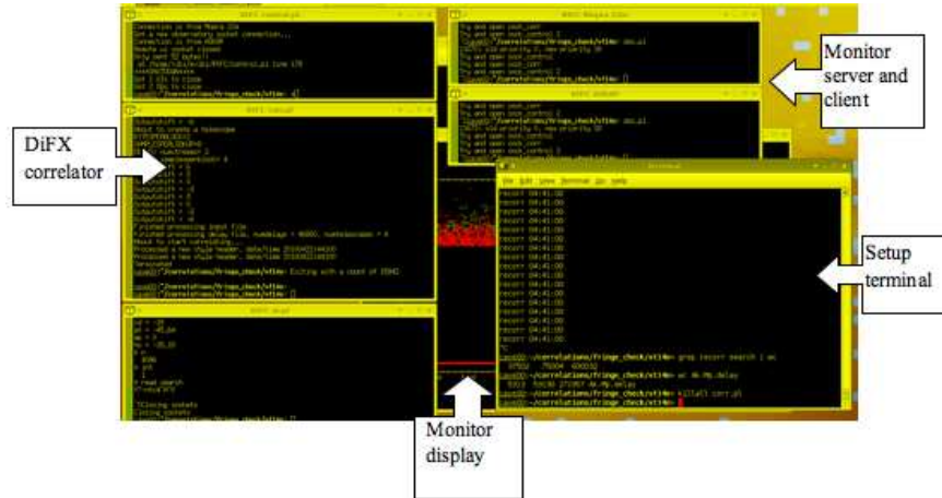
Figure 2.7: e-VLBI Software - The e-VLBI correlator and monitoring programs running during an e-VLBI experiment.
