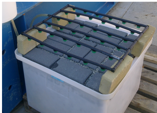
Figure 7: Test Rig 1 with Dripper Manifold (taken 14 July 2011, before water quality testing period began)
