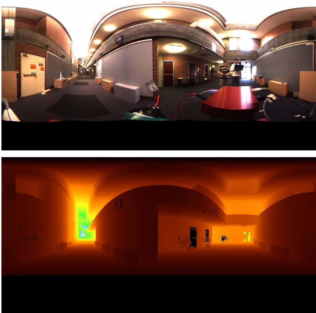
Figure 6.2 – Comparison of the image produced by the Ladybug omnidirectional camera (top) and the equivalent depth image produced from the associated laser point cloud.
