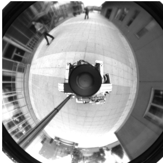
Figure 4.5 – An example image produced by a mirror based omnidirectional camera. Figure taken from Rituerto et al. [72].
