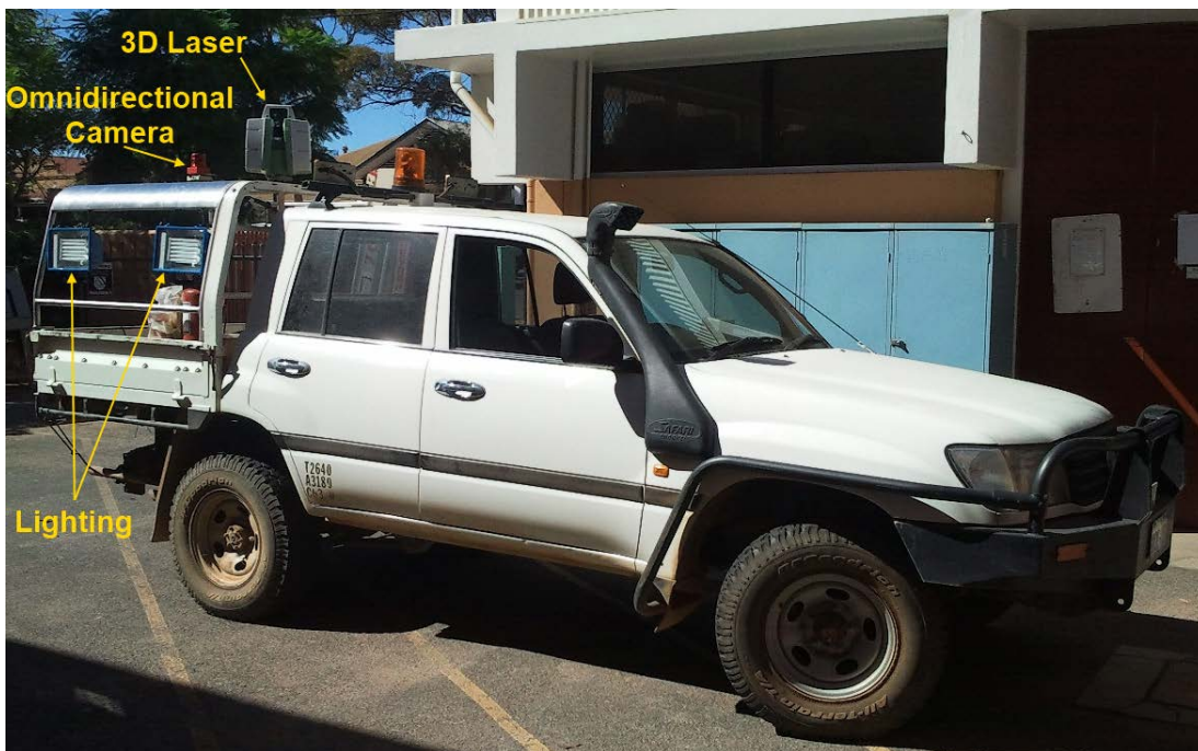
Figure 8.9 – The omnidirectional camera, 3D laser scanner and lighting mounted on a mine site certified vehicle.
