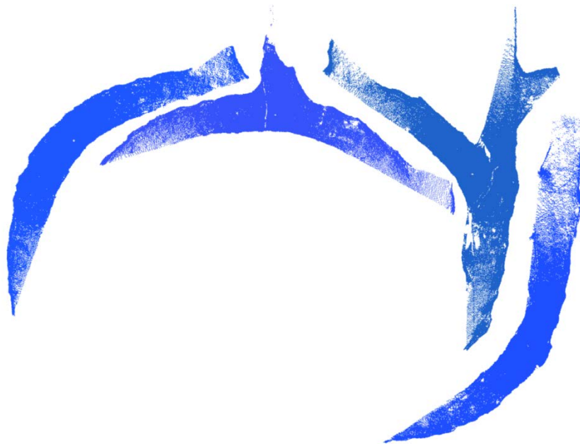
Figure 8.18 – The four laser scans comprising the spiral decline dataset. Alignment has been customized to give an idea of final fit.
