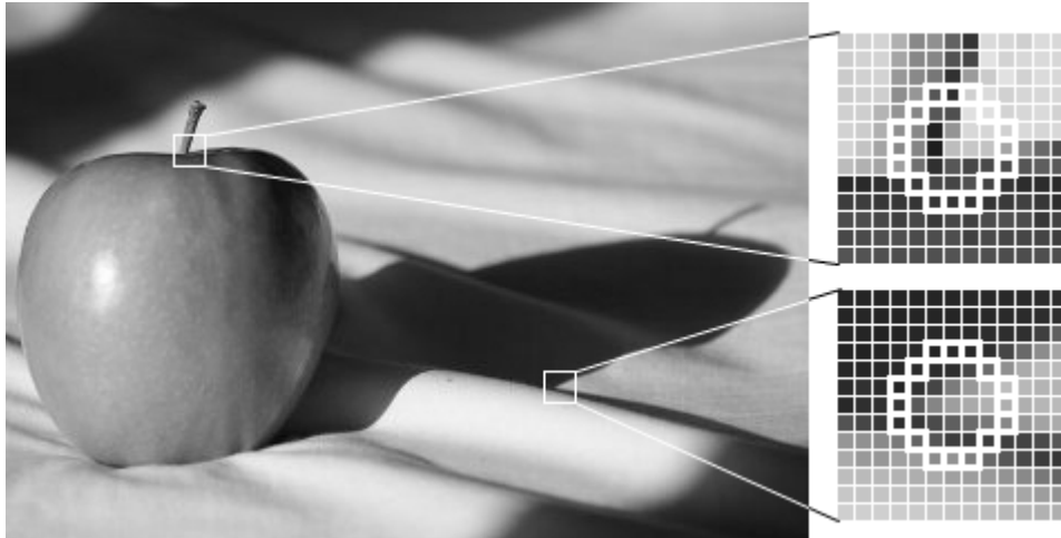
(c) Features on the monochrome image used by FAST corner detection.
