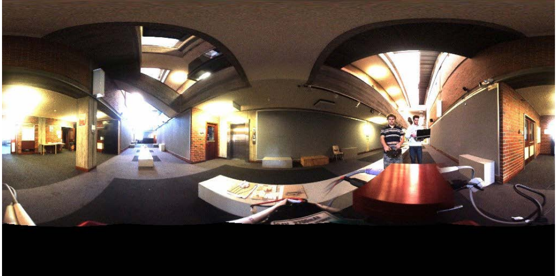
Figure 4.7 – Example panoramic image produced by the Point Grey Ladybug 2 omnidirectional camera. Note the masked section at the bottom of the image due to the cameras not covering the entire visual sphere.
