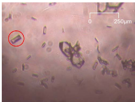
FIGURE 4.14: 400x optical microscope image showing an isolated prismatic crystal of \text{TiOSO}_4 \cdot \text{H}_2\text{O} (circled in red) produced after reaction for a further 72 hours.
