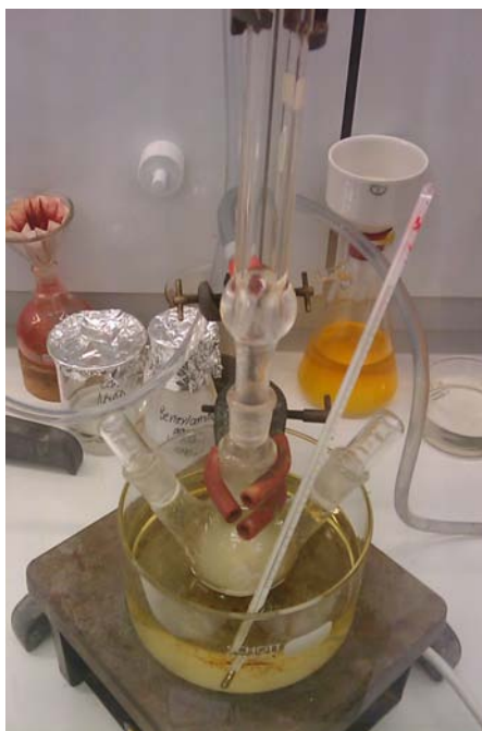
FIGURE 4.41: Photograph of the laboratory setup used to produce \text{TiOSO}_4 \cdot 2\text{D}_2\text{O} .
