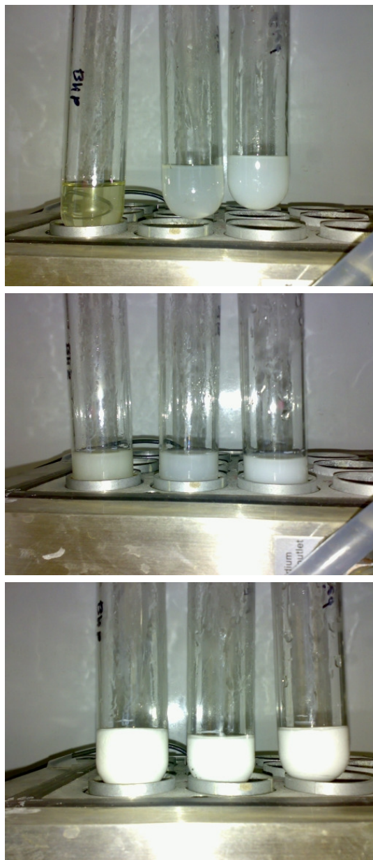
FIGURE 4.1: Photographs of the products of the reaction between 2.8g of \text{TiOSO}_4 produced from BHP Billiton (left), Sigma-Aldrich (middle) and Riedel-de Haen (right) \text{TiOSO}_4 \cdot 2\text{H}_2\text{O} precursor and 20mL of 400 \text{ gL}^{-1} \text{H}_2\text{SO}_4 at 110(\pm 5)^\circ\text{C} after 1 hour (top), 2.5 hours (middle), and 4 hours (bottom).
