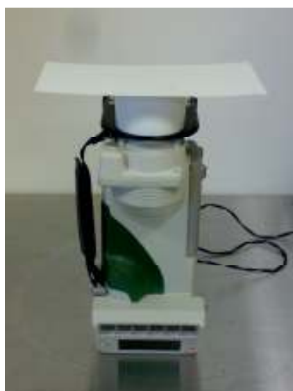
Figure 3-7: Measurement of colour on oil sample in Agtron cell covered by Leneta paper using a Minolta spectrophotometer
