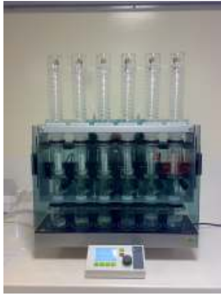
Figure 3-5: Buchi E-816 SOX Extraction Unit in operation
