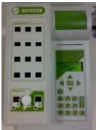
Figure 3-6: OxiTester assessing the peroxides value of an oil sample
