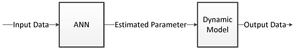
Figure 4.3: Structure of a serial hybrid model (Psichogios and Ungar 1992).
