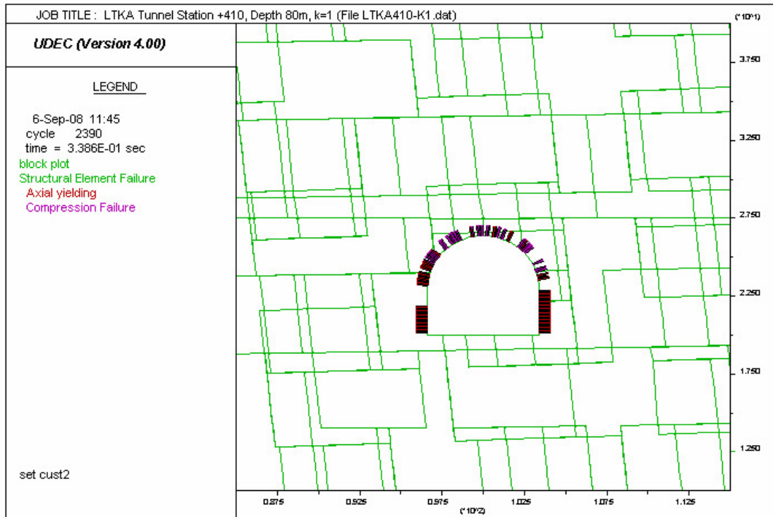
Figure C9 Failure of URF shotcrete at Sta. 410 m when k=1 (rock bolts not shown)
