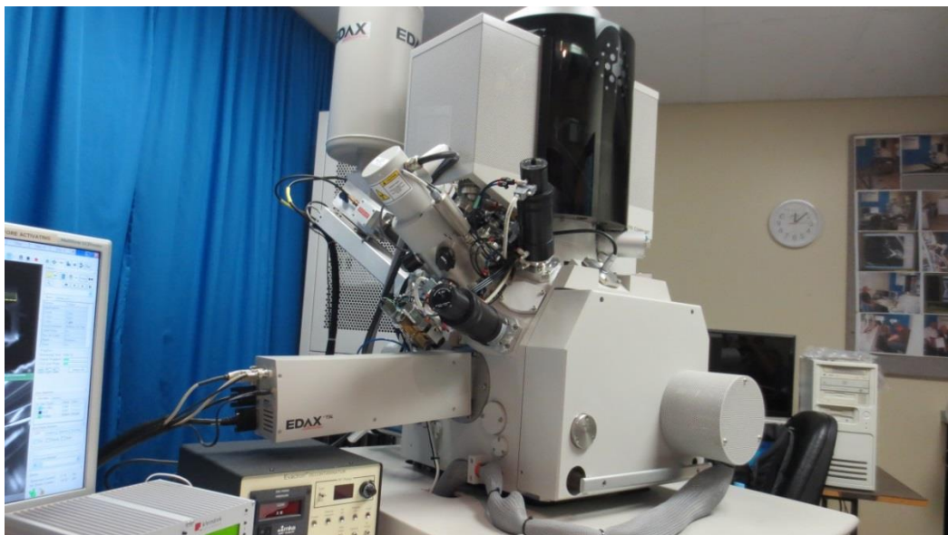
Figure 2-13: FIB/SEM Instrument used in the study to image the pore structure at sub-micron level
