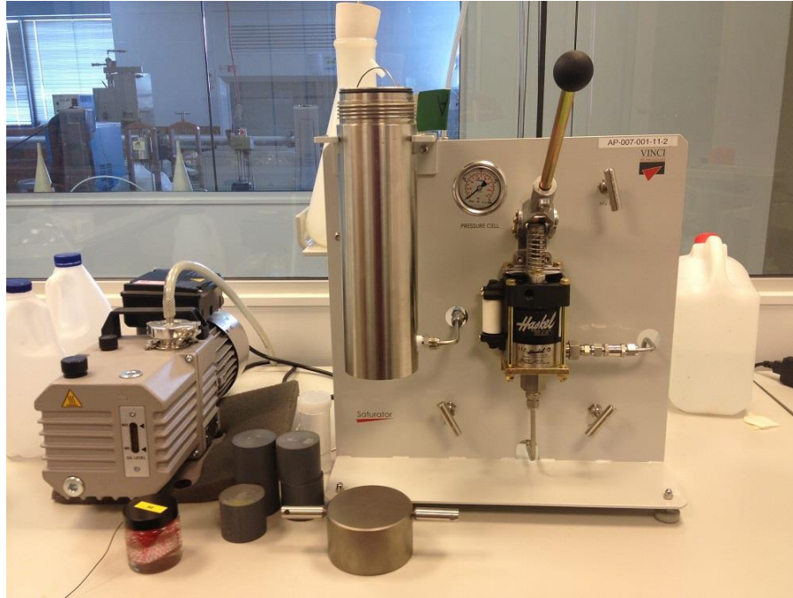
Figure 4-9: Instrument used to saturate the core plugs under 3.5 MPa hydrostatic pressure
