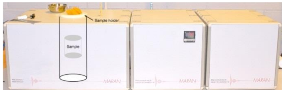
Figure 2-8: Low field Maran Ultra-Spectrometer 2 MHz used in this study to measure the amount of hydrogen protons in a given sample
