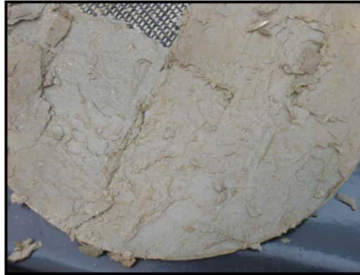
Figure 3.9 GCL with top layer removed
