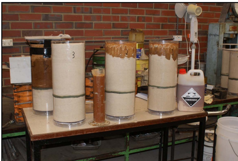
Figure 3.4 Filling of the Cylinders with Bayer Liquor
