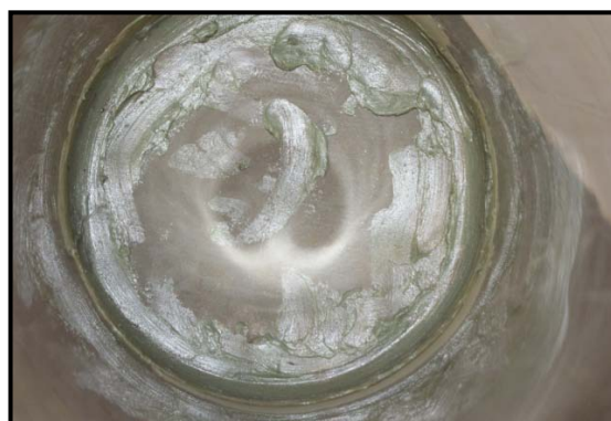
Figure 3.3 Mastic sealing the edges of the GCL to the cylinder
