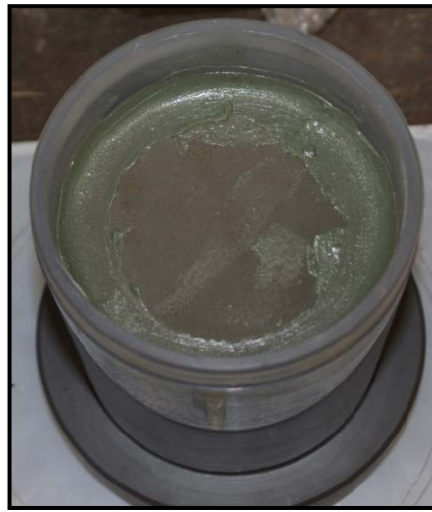
Figure 3.12 Sample in Test Rig with Mastic Seal
