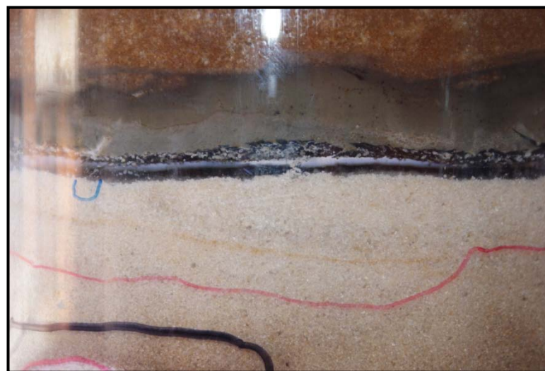
Figure 4.4 Cylinder 8 Completely Detached from Lower Layer
