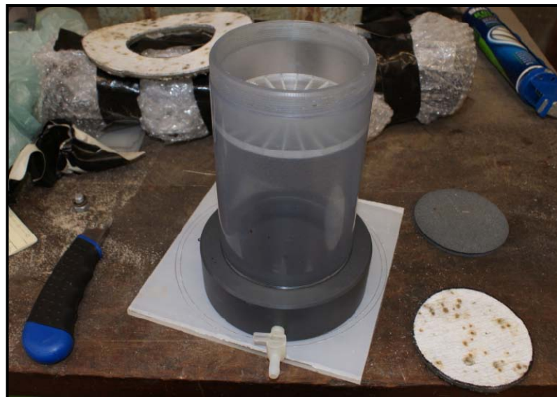
Figure 3.11 Lower Reservoir and bleed valve
