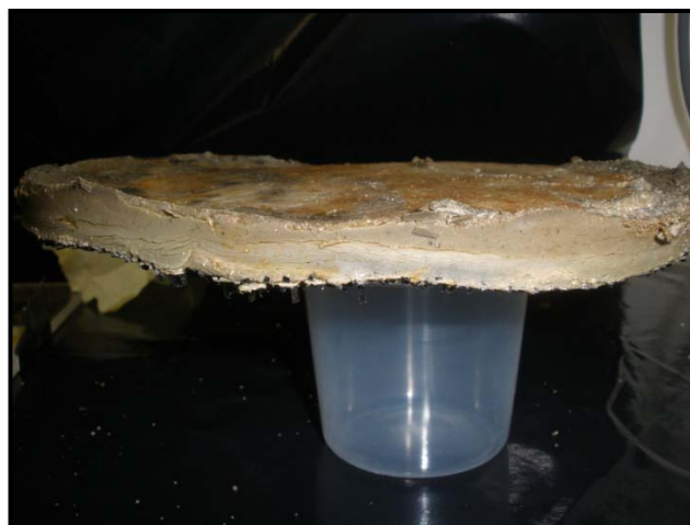
Figure 3.8 GCL Remove for Inspection
