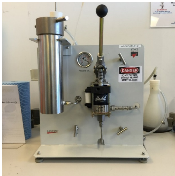
Figure 2-7 High-pressure saturator in the Department of Petroleum Engineering of Curtin University.
