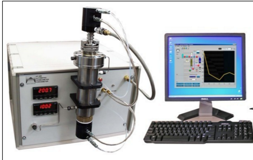
Figure 2-4 The automated porosimeter and permeameter (AP-608).
