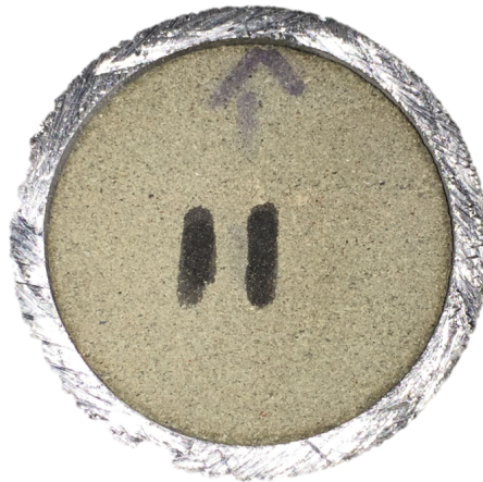
Figure 2-10 A sandstone sample confined by an aluminum tube in order to provide the confining pressure on the sample and reduce the sample's contact with air.
