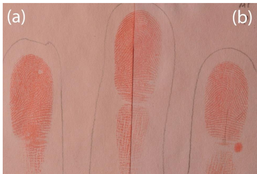
Figure 3.7: Fingerprints on white copy paper, treated with (a) Beaudoin's ORO for 60 minutes; and (b) ORO in propylene glycol for 15 minutes
