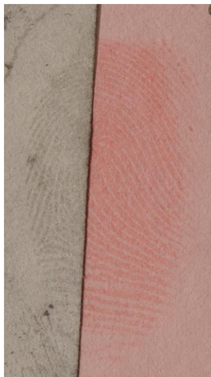
Figure 2.1: Example of a split fingerprint on white copy paper, treated with PD (left) and ORO (right)
