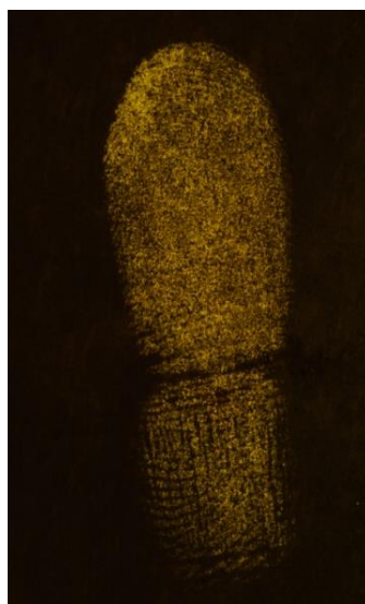
Figure 3.11: Charged fingerprint on white copy paper treated with 1 % Nile blue histological stain
