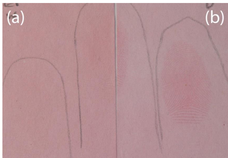
Figure 3.5: Fingermarks treated with ORO (a) after 1 hour immersion in deionised water; and (b) dry
