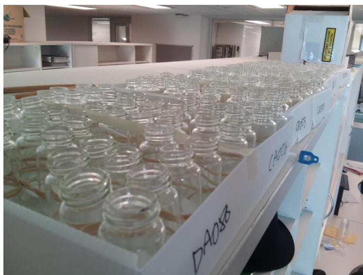
Figure 6.1: Arrangement of latent fingerprint samples stored in open vials over a 28 day period
