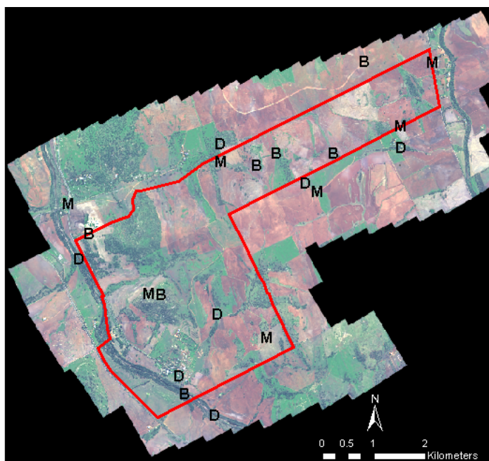
Figure 3.6 Geographic distribution of target locations overlaid on reference image (DMSI June 2004). Where B, represents bright targets; M, the midrange targets; and D, represents dark targets
