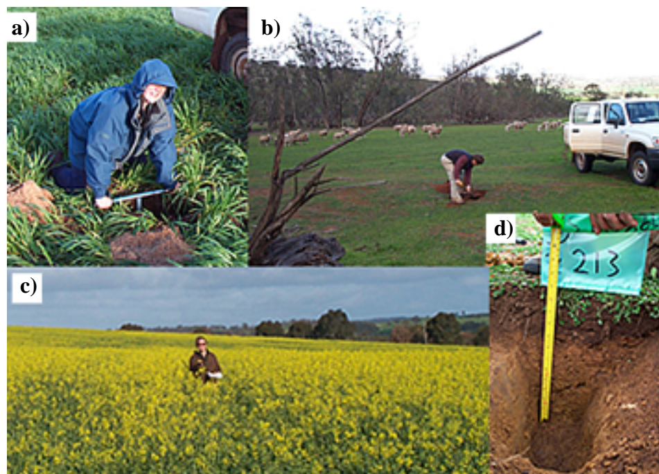
Figure 4.7 Soil sampling Field Data Collection. a) Auguring soil pit to maximum depth of 80cm, b) Digging soil pit, c) Recording the dGPS position of soil sampling point, d) Soil sample point 213, soil pit
