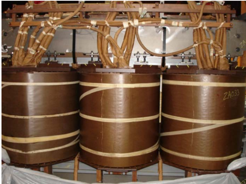
Figure 3-6. Layer winding type[54]
