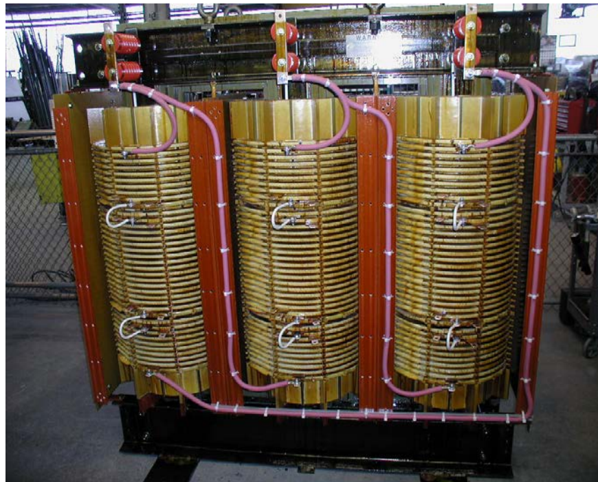
Figure 3-4. Shell type transformers[54]
