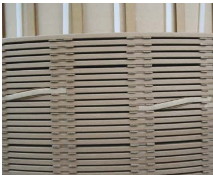
Figure 3-8 Disk winding type[54]
