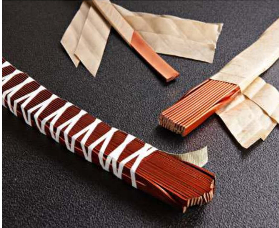
3-5. Rectangular shape conductor[54]
