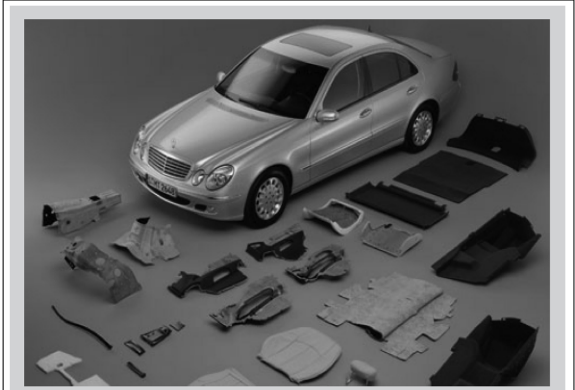
Figure 2.10: Fifty components made from natural fibres which are part of Mercedes-Benz's E series of cars (Holbery and Houston, 2006).
