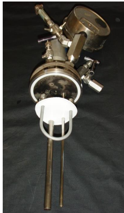
Figure 6: Early version of the TOL corrosion test set up
