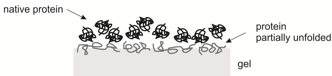
Figure 4.3.17. Diagram of the proposed multilayer formed onto the hydrophobic gel. Note that the electrolyte present in the gel which interacts with the protein is not illustrated in this diagram.
