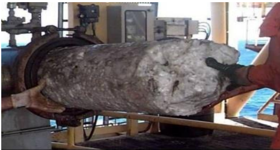
Figure 2.13: Subsea gas pipeline plugged by hydrate (Lorenzo, 2009)
