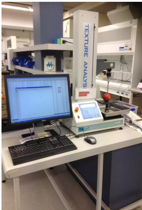
Figure 3.4. Determination of sample fruit firmness and graphical presentation of firmness profile of sample fruit using texture profile analyzer (TPA).
