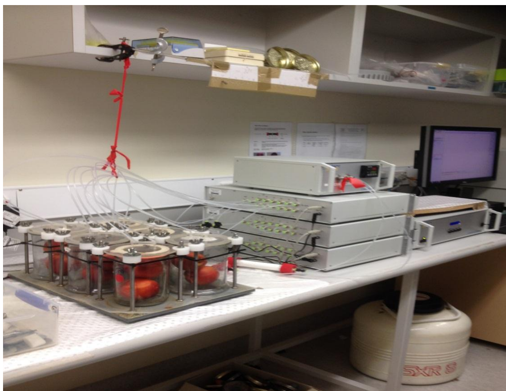
Figure 3.2. Determination of ethylene production from the sample fruit by using ETD 300 ethylene detector.
