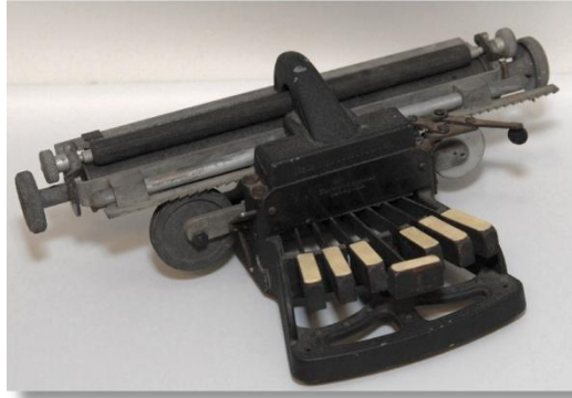
Figure 3.3: Photo of the Marburg Braille Writer (The New York Institute for Special Education 2008)
