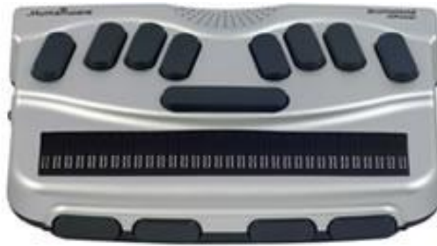
Figure 3.15: BrailleNote Empower with 32 Braille Cell Display (Humanware, 2008a)
