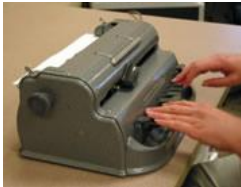
Figure 3.5: Perkins Machine (Adaptive Technology Center 2008)
