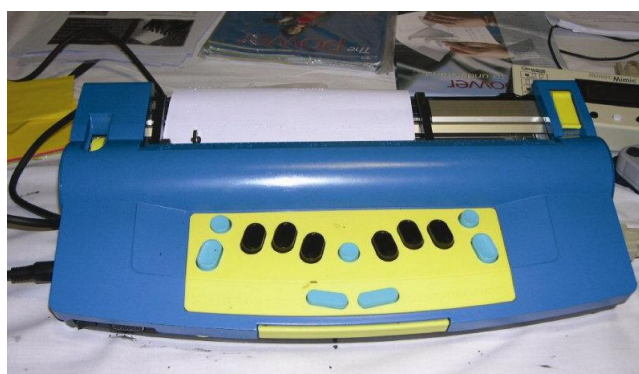
Figure 3.10: Mountbatten Brailler System (Quantum Technology, 2008)
