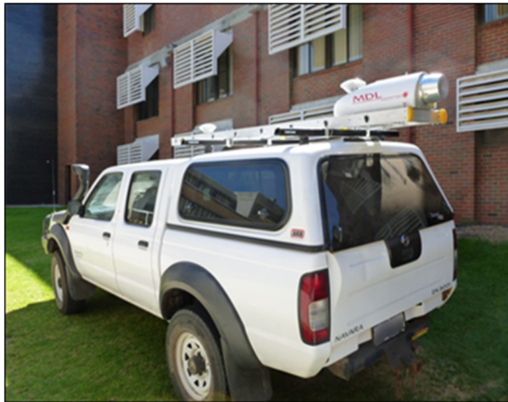
Figure 1.1 Mobile mapping vehicle with onboard sensors (Courtesy, Department of Spatial Sciences, Curtin University).
