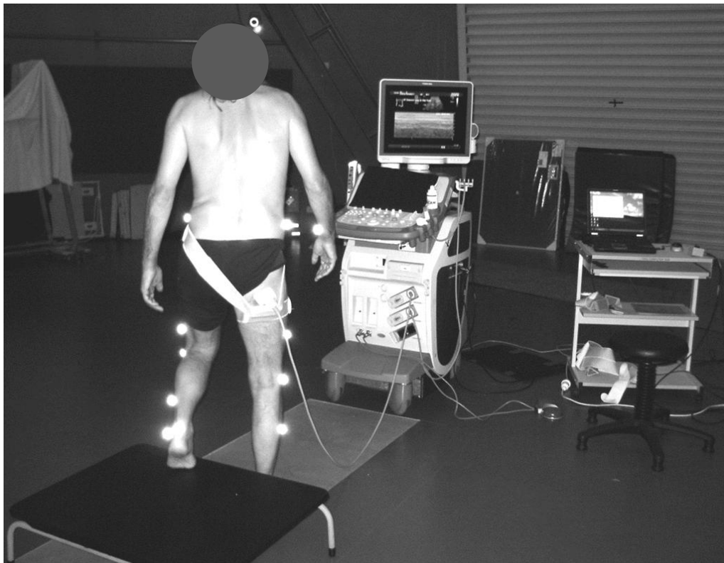
Figure 8.2. Subject performing a step down onto a floor-inbuilt force platform (US transducer here on the hip extensors for another investigation).
