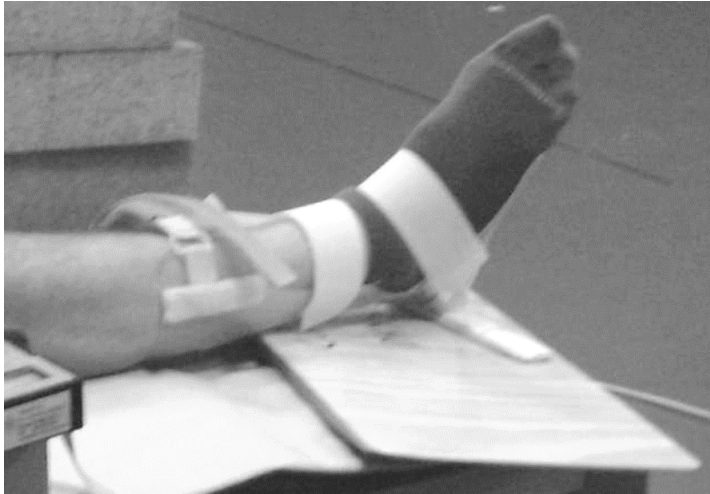
Figure 3.11. Leg rotation was secured by a splint around the calf, which was positioned on a sliding board.
