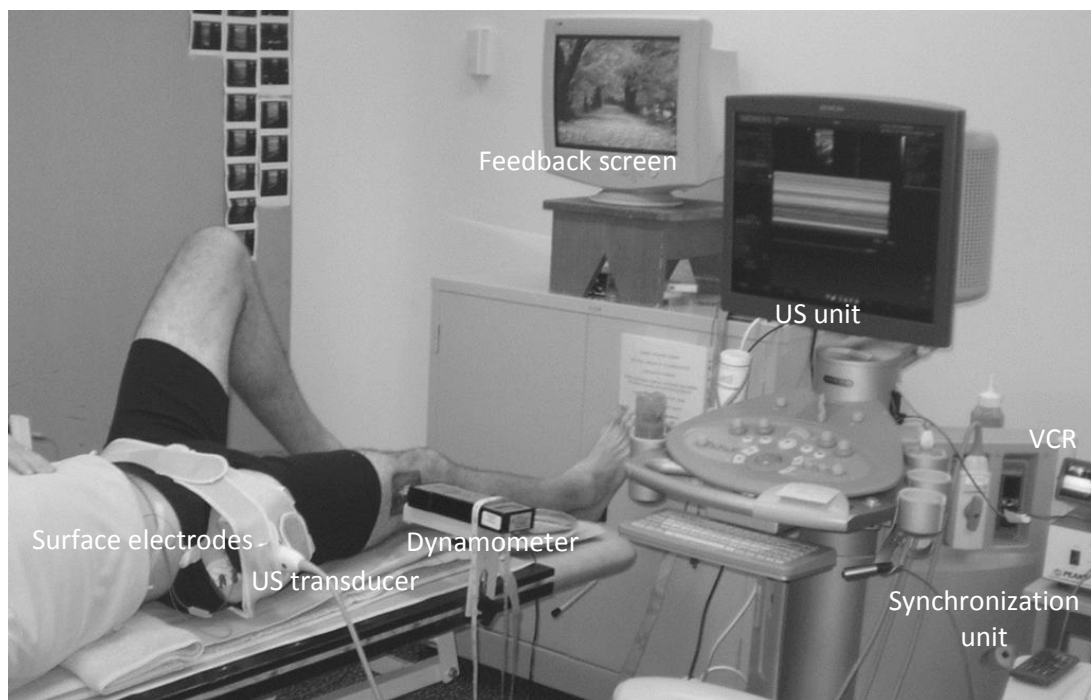
Figure 3.8. Setup One: isometric hip abduction recorded by dynamometry, surface EMG and US.
