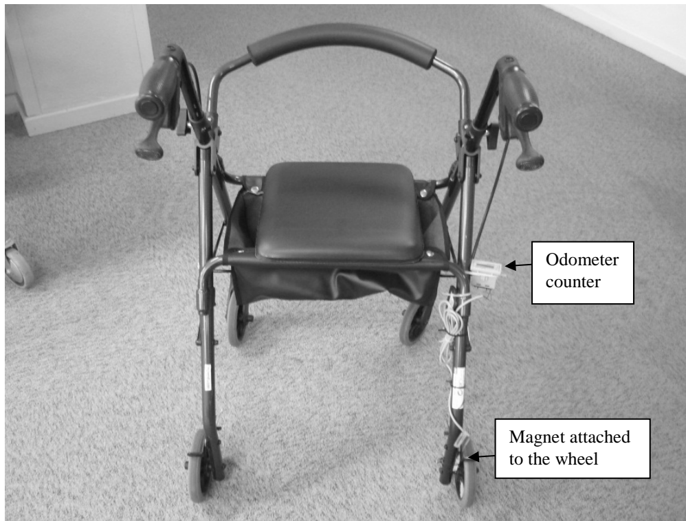
Figure 4-3: A wheeled walker with a magnetic odometer attached to a rear wheel.
