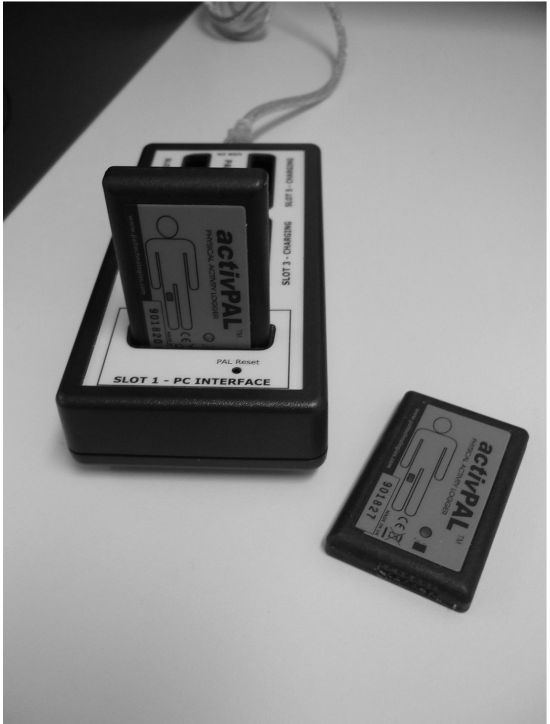
Figure 3-2: ActiPAL™ and the USB docking station.
