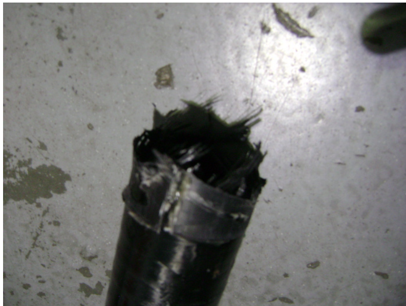
Figure 5-40: Carbon/epoxy failure during tensile testing
