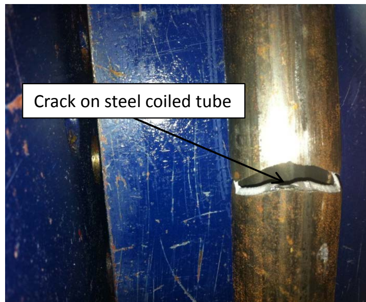
Appendix 5.1: Tube 1 Fracture failure
