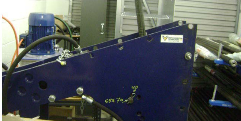
Figure 5-33: Fatigue testing of carbon/epoxy tube
