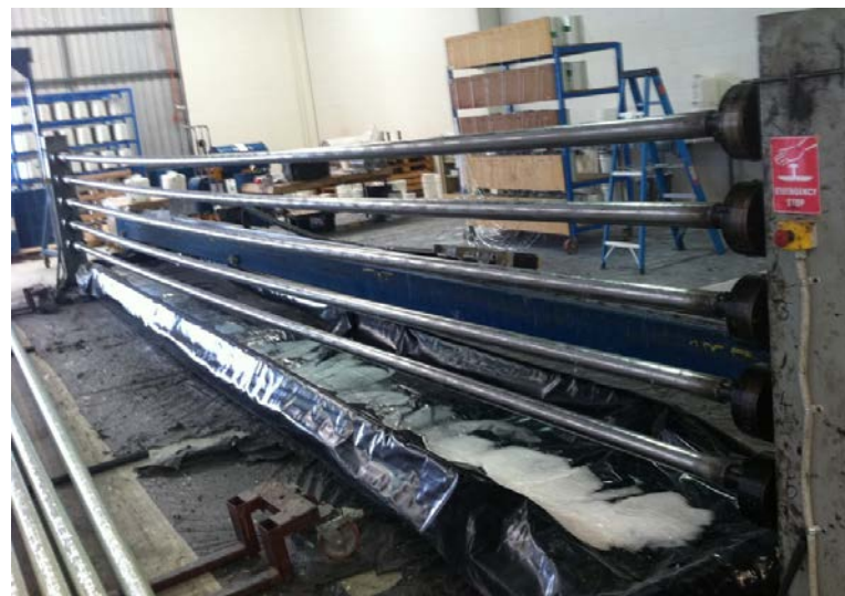
Figure 5-31: Filament winding machine (Courtesy of Teakle Composites)
