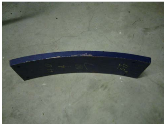
Figure 3-9 40 inch (1016mm)n radius steel bending form
