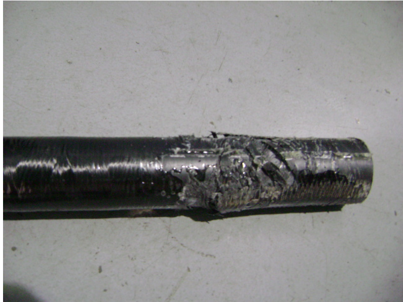
Figure 5-39: Fibre breakage on carbon/epoxy tube during tensile testing (tube 1A)
