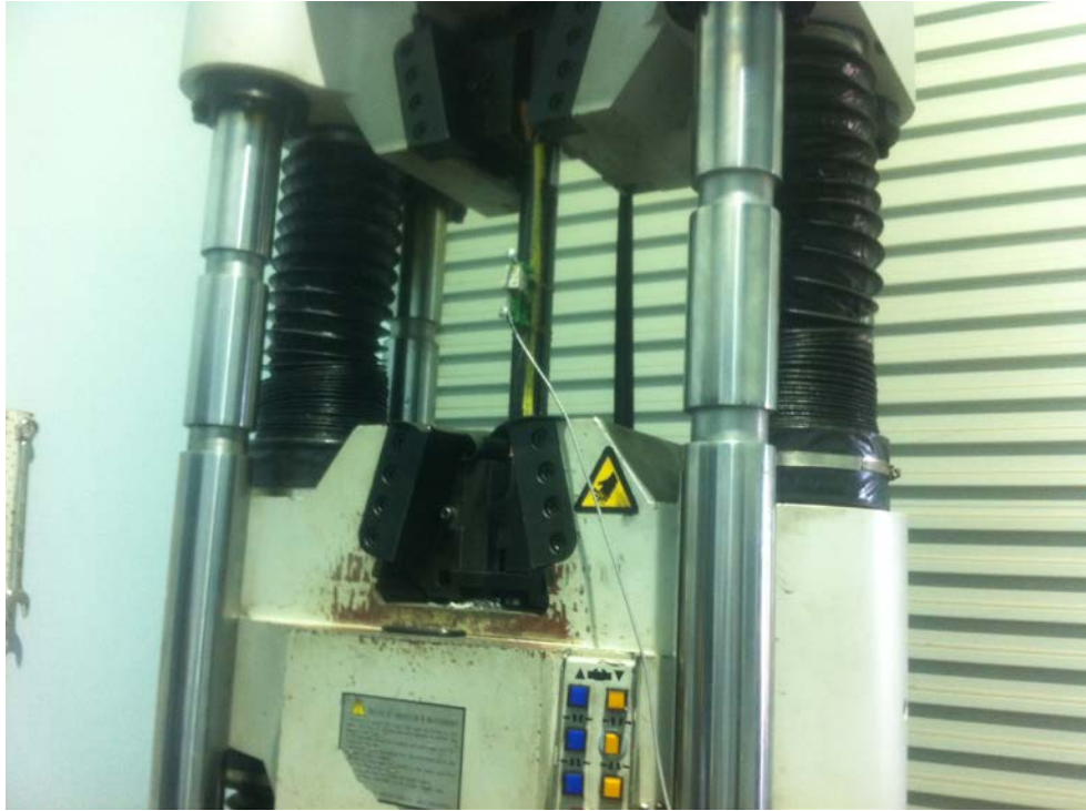
Figure 5-37: Experimental set up of carbon/epoxy tube tensile test
