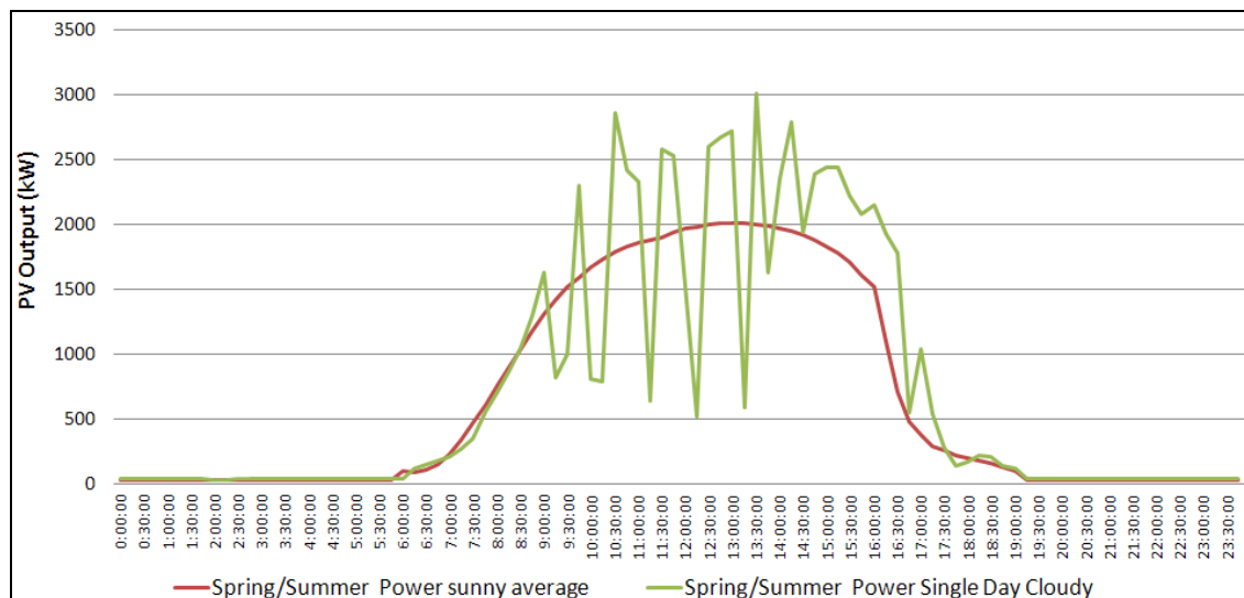
Figure 6. 7: Single day and average output of a 2.5kW PV system with a 5kW rated inverter, data taken at 15 minute intervals [1]
