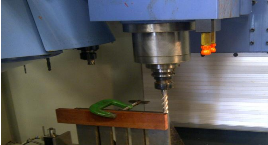
Figure 8.4 CNC cutter finding Z origin
