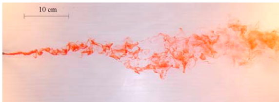
Fig. 1. Flow visualization of the chemical plume in a controlled turbulent flow. The view is from above, with the flow moving from left to right.
