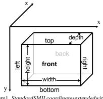
Figure 1. Standard SMIL coordinates extended with front, depth, and back coordinates.
