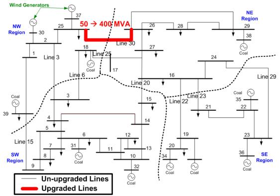
Figure 84: Overview of the transmission upgrades required in the DSR case.
