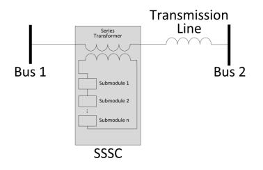
Figure 28: Static synchronous series compensator (SSSC).
