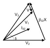
Figure 23: Phasor diagram with a series capacitive controller installed at the Bus One side of the transmission line.
