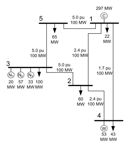
Figure 78: Base case system. The line values represent the admittance and max power flow. The generator types are designated by C, G, and W for coal, CCGT natural gas, and wind respectively. The generator values indicate the generator capacity. The load values indicate the peak load.
