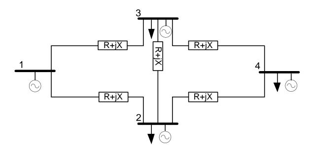
Figure 57: Four-bus system for study of centralized-localized IPF control.
