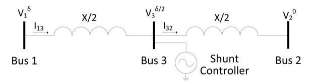
Figure 13: Connection of a shunt controller at the midpoint of the transmission line.
