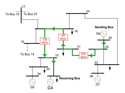
Figure 48: Locations and ratings of BTB converter to realize a 20 MW IPF transaction.
