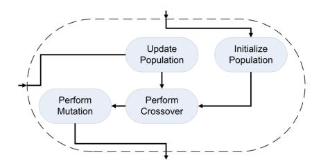
Figure 76: Flowchart for the genetic algorithm.
