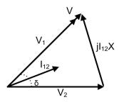
Figure 12: Phasor diagram with a shunt controller installed at Bus One.
