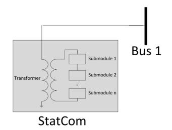
Figure 20: Modular multilevel static synchronous compensator (StatCom).
