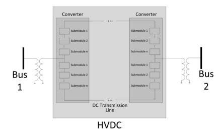
Figure 41: High voltage DC (HVDC) transmission system using modular multilevel converters.
