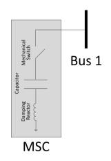
Figure 15: Mechanically switched capacitor (MSC).
