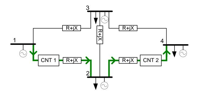
Figure 60: Test-system with CNTs installed to execute transactions along one path.
