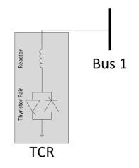
Figure 18: Thyristor controlled reactor (TCR).
