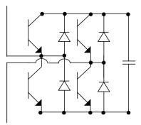
Figure 21: Submodule of a modular multilevel StatCom.
