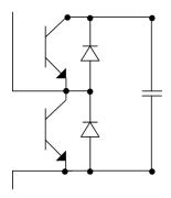
Figure 42: Submodule of a modular multilevel HVDC.
