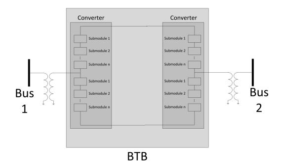
Figure 43: Back-to-back converter (BTB).
