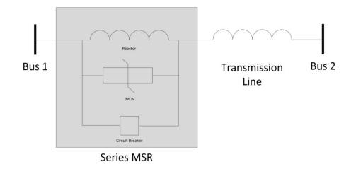
Figure 25: Series mechanically switched reactor (MSR).
