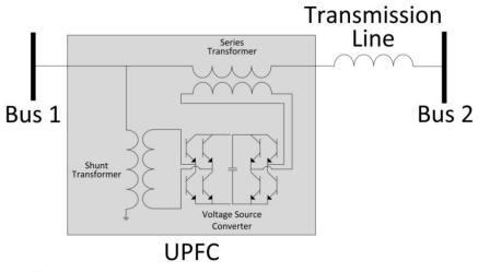
Figure 32: Unified power flow controller (UPFC).
