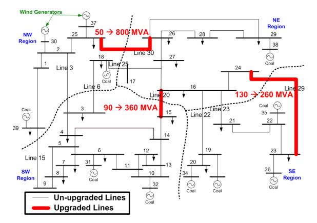
Figure 83: Overview of transmission upgrades required in the BAU case.
