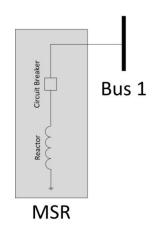
Figure 16: Mechanically switched reactor (MSR).
