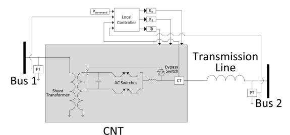
Figure 59: CNT and local controller embedded in a transmission line.
