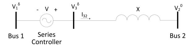
Figure 22: Connection of a series controller at the Bus One side of the transmission line.
