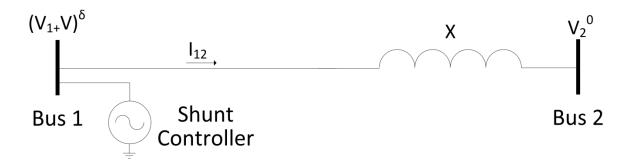
Figure 11: Connection of a shunt controller at Bus One.
