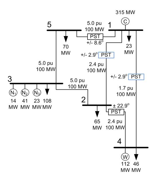
Figure 81: System topology, generation capacity and peak load at the end of the second decade under the revised centralized transmission planning framework. Transmission assets added in the second decade are shown in blue.
