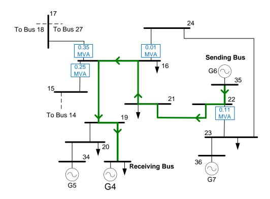
Figure 49: Locations and ratings of CNT converters to realize a 20 MW IPF transaction.
