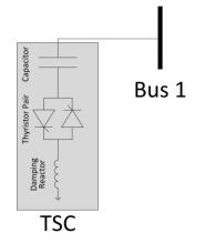
Figure 17: Thyristor switched capacitor (TSC).
