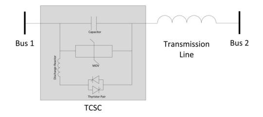
Figure 27: Thyristor controlled series capacitor (TCSC).
