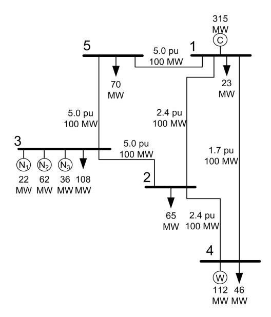
Figure 74: System topology, generation capacity and load for the CSCOPF demonstration cases.
