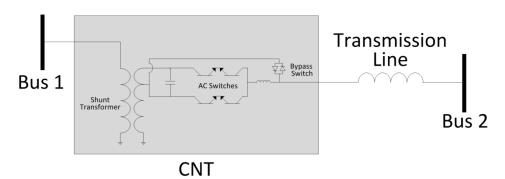
Figure 34: Controllable network transformer (CNT).
