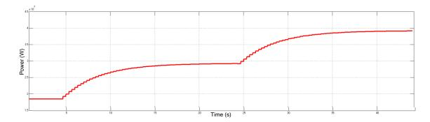
Figure 61: Power flow through Line<sub>1-2</sub> of the IPF transaction path.
