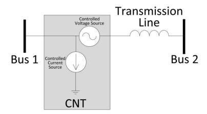
Figure 58: CNT model using voltage and current sources.
