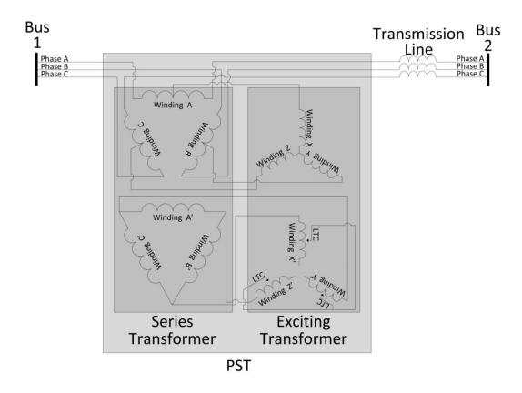
Figure 37: Three-phase diagram of a two core phase-shifting transformer (PST).
