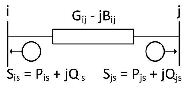
Figure 82: Model of a PF converter connected to Line  $_{i-j}$  per the power injection method.
