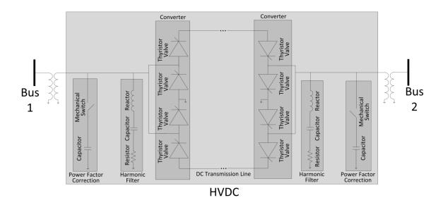
Figure 40: High voltage DC (HVDC) transmission system using line commutated converters.
