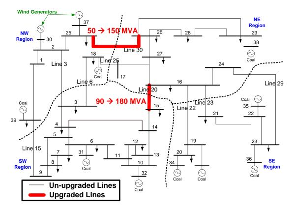
Figure 85: Overview of transmission upgrades required in the IPF control case.
