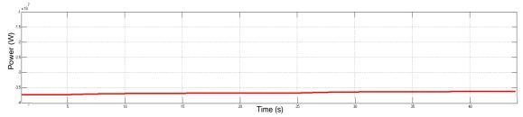
Figure 63: Power flow through Line<sub>3-1</sub>, which is not part of the IPF transaction path.
