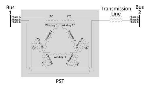
Figure 36: Three-phase diagram of a single core phase-shifting transformer (PST).
