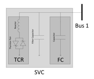
Figure 19: Static VAr compensator (SVC).
