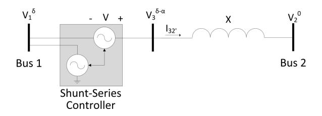
Figure 30: Connection of a shunt-series controller to the power line.
