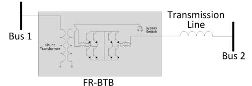
Figure 35: Fractionally-rated back-to-back (FR-BTB).
