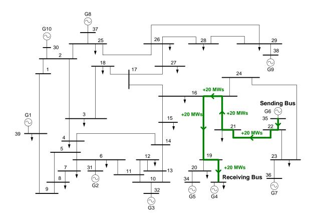
Figure 46: IEEE 39-bus system with desired incremental transaction shown in green.
