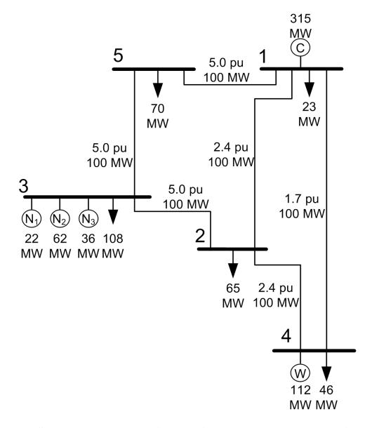
Figure 79: System topology, generation capacity and peak load at the end of the second decade under the centralized transmission planning process.
