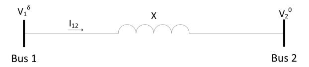
Figure 9: Two-bus system connected by a single transmission line.
