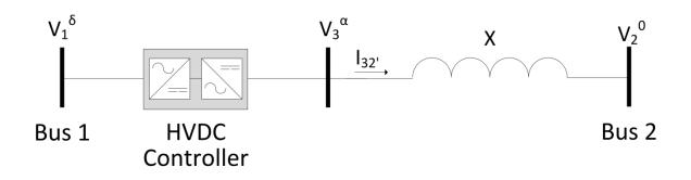
Figure 38: Phasor diagram of an HVDC controller connected between Bus One and Bus Three.
