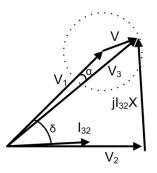
Figure 31: Phasor diagram of a shunt-series controller connected to Bus One and the line between Bus One and Bus Two.
