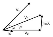
Figure 39: Phasor diagram of an HVDC controller connected to Bus One and supplying the line between Bus Three and Bus Two.
