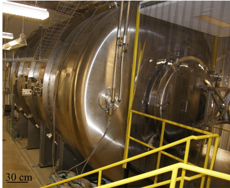
Figure 51: The VTF-2 vacuum facility at the Georgia Tech HPEPL with the walk-in door shown on the right.
