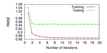
**Figure 14:** Performance measured by RMSE with respect to the number of iterations on MovieLens data set.
