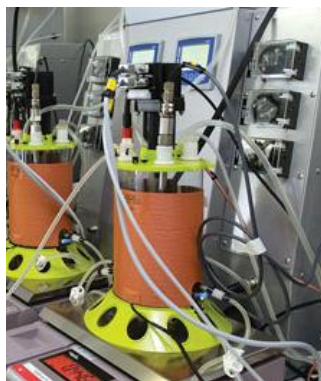
Fig. 4: Typical mammalian cell culture process in a small-scale bioreactor. Source: Figure taken at Merck Site Martillac.
