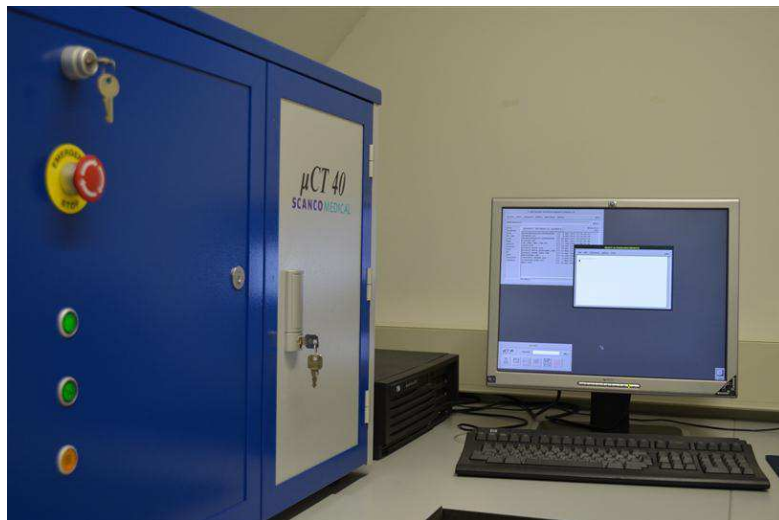
Figure 3.2 (A) a sample was put on the sample holder in a humid environment using Parafilm (Parafilm M, Pechiney Plastic Packaging, Chicago, USA) to seal the upper side of the sample holder in order to prevent the desiccation of the tooth. (B) A high resolution X-ray micro-computed tomography ( \mu CT 40, Scanco Medical AG, Basserdorf, Switzerland) was used for this investigation.
