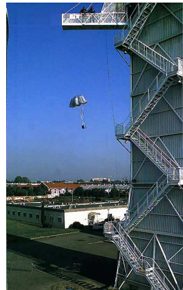
Figure 9. Drop of a small hemispherical parachute.
