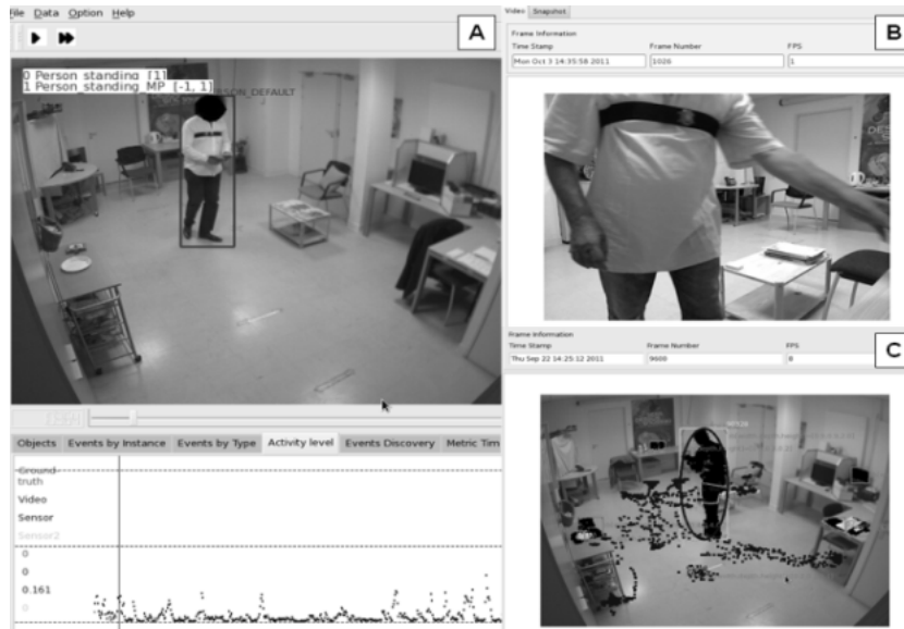
Fig. 8 Participant’ activities by the point of view of different sensors: (A) RGB camera view and actimetry provided the inertial sensor (the bottom of image A); (B) RGB-D camera view of participant, which shows the inertial sensor worn by the participant; and (C) Drawn points on the ground represent the trajectory information of the participant during the experimentation.
