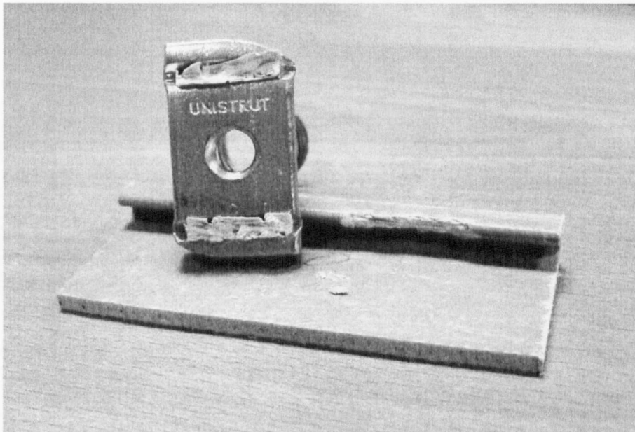
Figure 3.15: Material damage to GS1 shape after 5 mm slip with standard nut and bolt \geq 15 Nm
