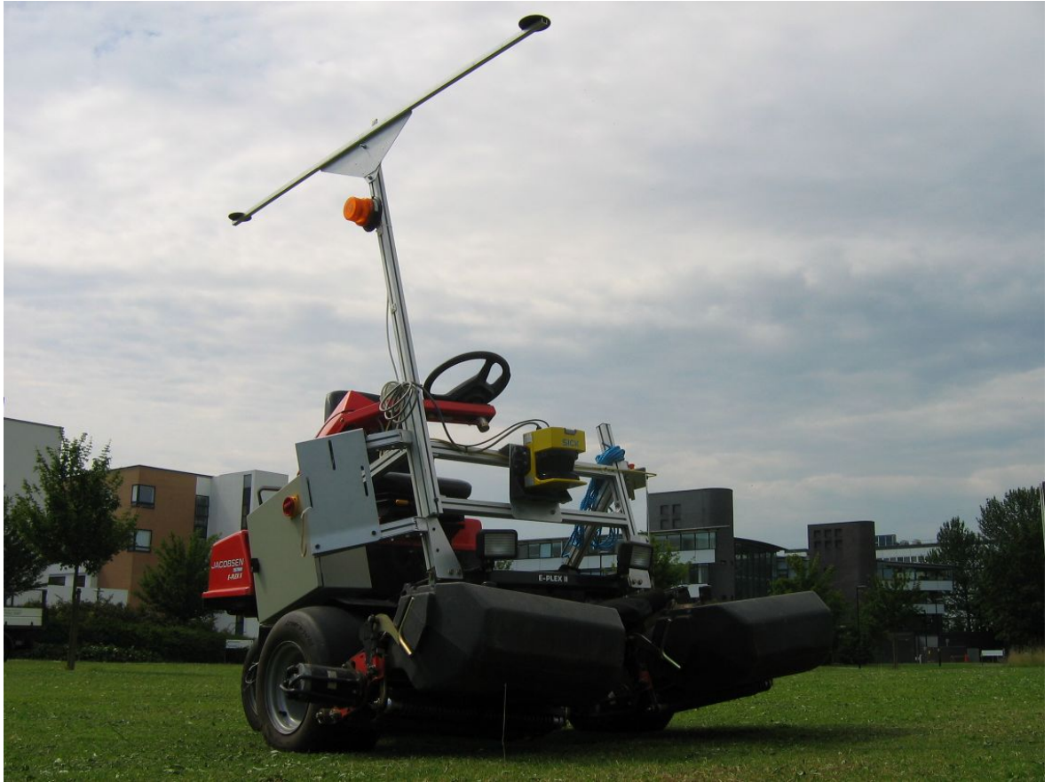
Figure 5.3: Test vehicle fitted with two single frequency GPS receivers 1.9 metres apart, north to south.
