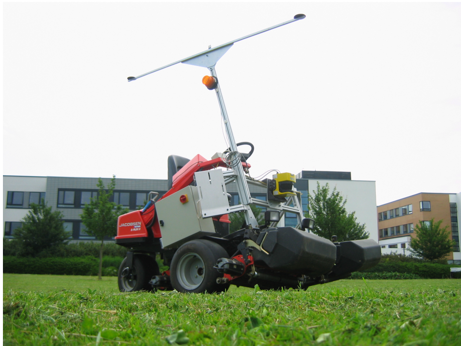
Figure 2.1: E-Plex II mower fitted with GPS, LIDAR and control electronics.
