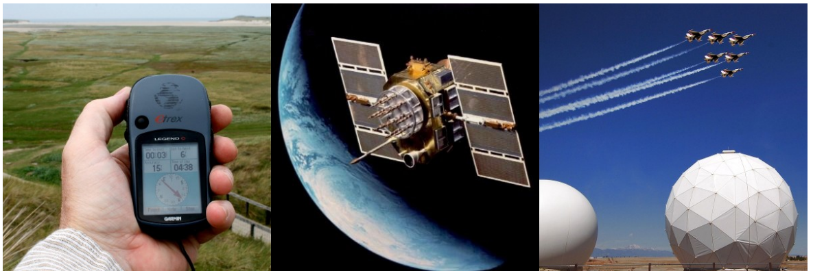
Figure 3.1: GPS is comprised of three segments; the user segment (left), the space segment (centre) and the control segment (right).
