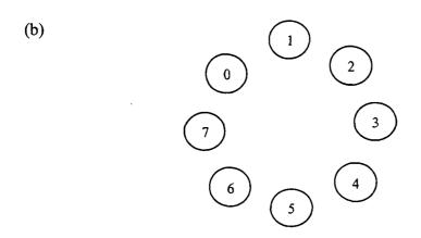
Consider the ring-based election algorithm. Two processes, 2 and 5, discover simultaneously that the previous coordinator, process 7, has crashed. Hence both processes 2 and 5 start an election simultaneously.
