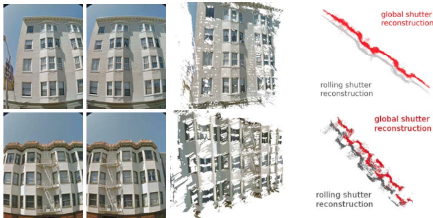
Figure 8. Real world reconstruction of the Oak street (top) and Fillmore street (bottom) data sets show systematic differences in bird's eye view (right column).
