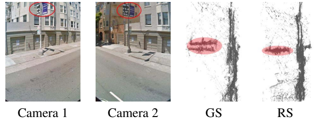
Figure 7. Left, sample input image of two cameras mounted on a car. We apply GS and RS stereo on both camera streams independently and fuse the resulting models into a single coordinate frame. Right, bird's eye view of GS and RS reconstruction. Note how the pole aligns in the RS reconstruction, while in the GS reconstruction it appears as two different poles.
