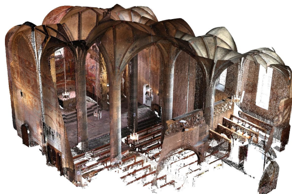
Figure 1: Cut through a 3D models obtained by our algorithm from 5 individual scans (CHURCH dataset). We achieve entirely automatic registration of arbitrary geometry from largely different viewpoints by exploiting depth and image data jointly.
