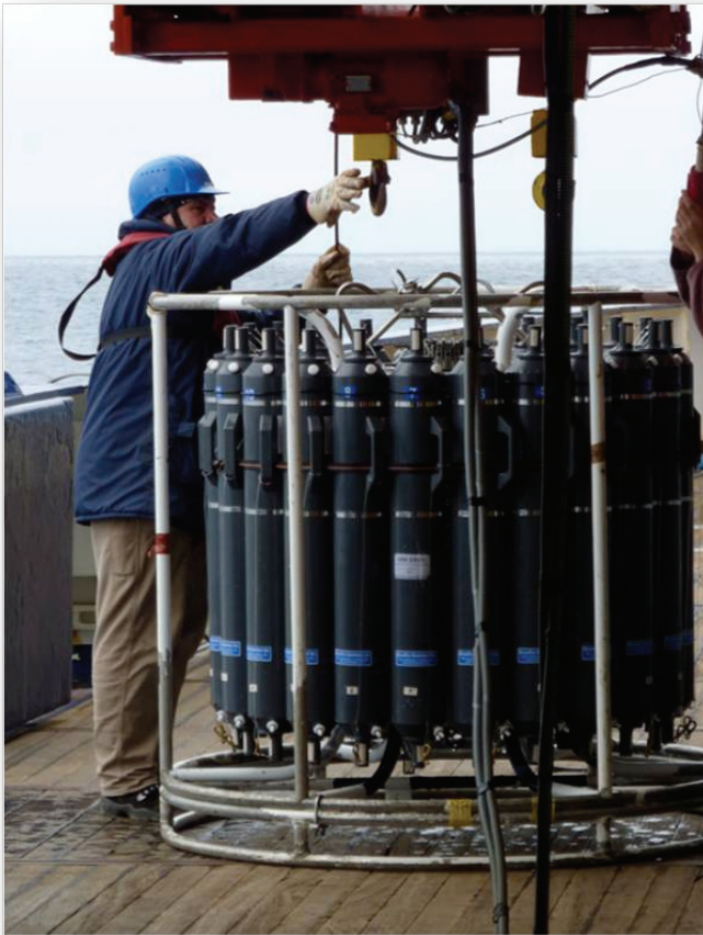
Fig. 3.1.1: Recovery of the CTD/Rosette at HAUSGARTEN observatory
