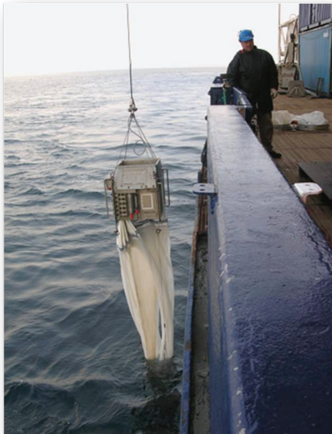
Fig. 4.1: Deployment of the Multi net to collect mesozooplankton in the HAUSGARTEN area
