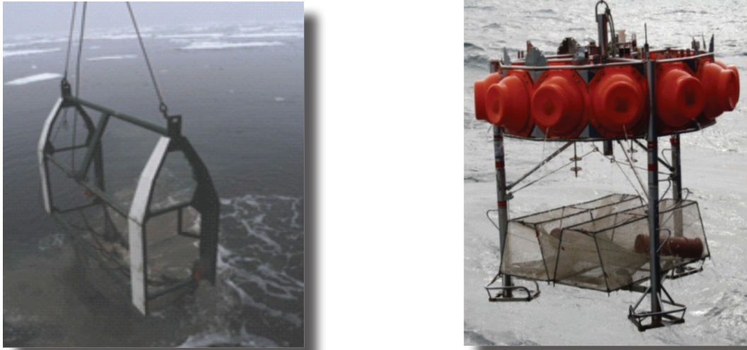
Fig. 3.7.2: Agassiz trawl retrieved at N-4 (left) and baited trap lander recovered at HG-IV (right)
