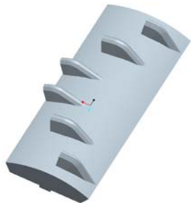
Figure 1. Three dimensional entity graph of the toothed plate.
