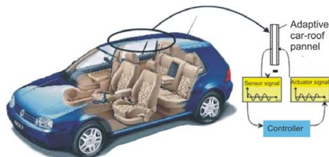
Fig. 1 Composite material architecture of an adaptive car-roof
