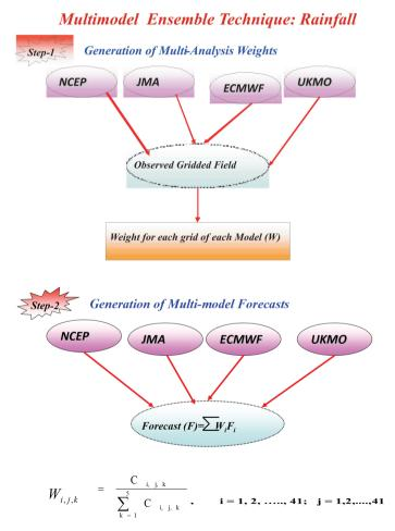
Figure 1. A schematic diagram showing the MME approach.
