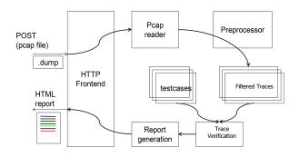
Slika 7. Passive testing trace verification tool
