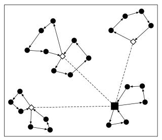
Figure 5 – Example of Two-Echelon Vehicle Routing Problem without inter-satellite communication
